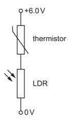
The thermistor has a resistance of  $6000\,\Omega$  in a cold room and  $1000\,\Omega$  in a warm room. The LDR has a resistance of  $2000\,\Omega$  in dim light and  $500\,\Omega$  in bright light.
